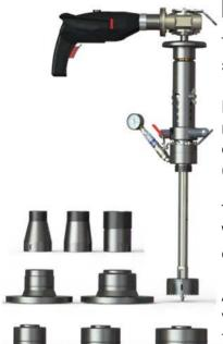
The lightweight and robust TONISCO B30 Hot Tap Machine Set is designed for making connections to pipelines, tanks, and plant piping.
