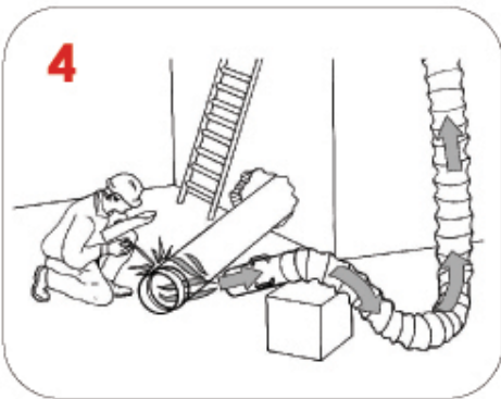
Suction of welding fumes in indoor works
