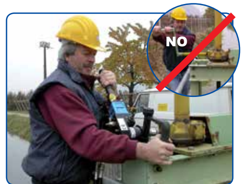
AH15 used in operating opening/closing the gates of irrigation canals
