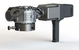
TONISCO B40 Electric drive unit is designed to be used as the turning force of TONISCO B40 Hot Tap Machine when making DN100-500 (4" - 20") hot tapping works. It has a variety of different speed selections to ensure the best cutting speed for different cutter sizes.
