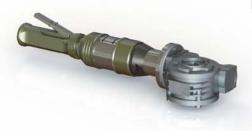
TONISCO Jr. Pneumatic drive unit is designed to be used as the turning force of TONISCO Jr. Hot Tap Machine when making DN20-100 (3/4" - 4") hot tapping works. It is a reliable and compact pneumatic drive unit with easy-to-use safety clutch.
